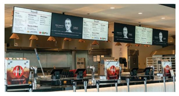
inches to 82 inches—with the majority of them being the 65-inch QM65H model; all of them have an integrated SoC player. The displays are mounted using a variety of mounts from SnapAV, Crimson AV and Solid Mounts. Fitzpatrick said the variety of applications—from menu boards to retail—dictated the need for many types of mounts.
